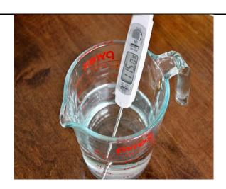
3. Insert the probe into the sample and wait for the measurement to become steady, which indicates the meter has reached equilibrium.
