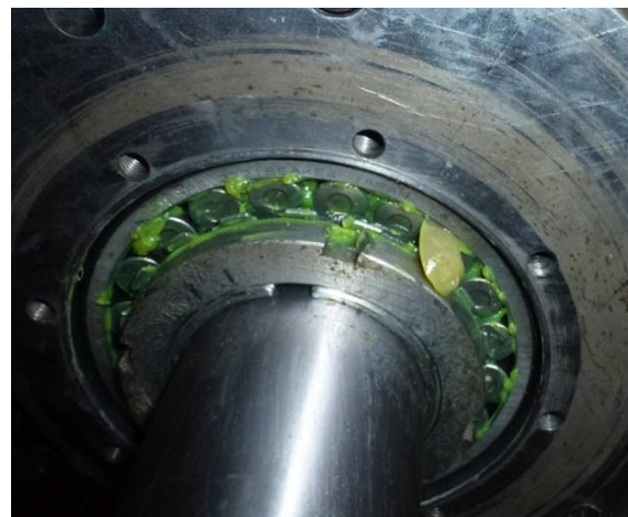
Figure 8: Properly lubricated and maintained bearing. Improvement of maintenance by installing vibration and temperature sensors.
