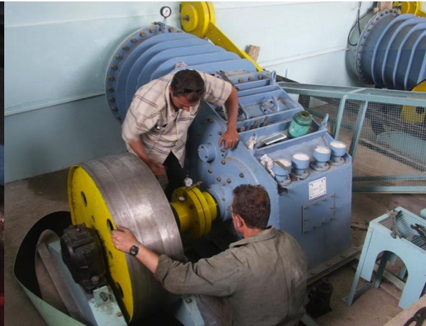
Figure 39: Checking alignment of the flexible coupling on a flat belt drive transmission driven with a crossflow turbine.
