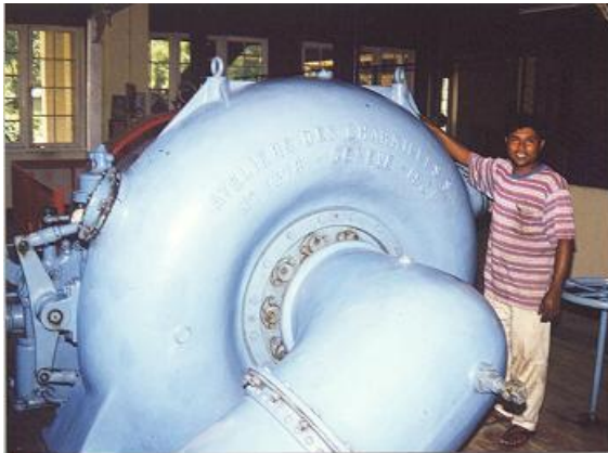
Figure 59: A horizontal shaft francis turbine.
