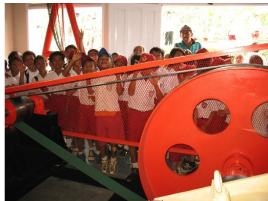
Figure 72: A high efficiency flat belt drive. The step-up ratio is high indicating low head / speed.
