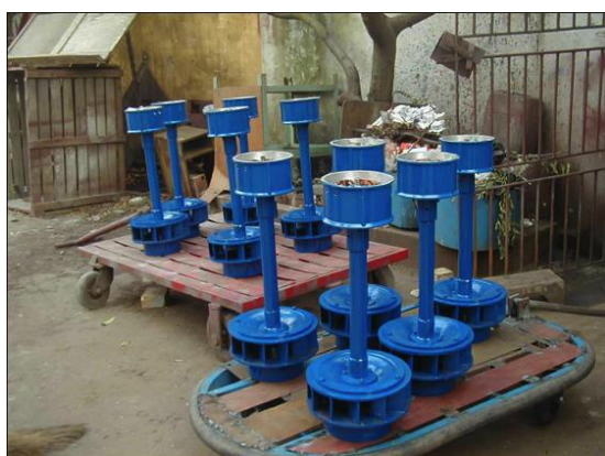
Figure 5: Pico hydro turbine units are installed widespread in SE Asia for producing a few watts for lighting individual houses.
