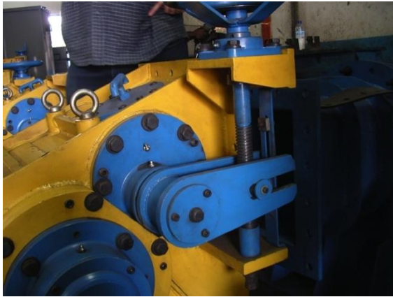
Figure 26: View of the guide vane adjusting mechanism on a cross flow turbine.
