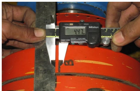
Figure 37: Checking the free movement of the rubbers of a flexible drive coupling.
