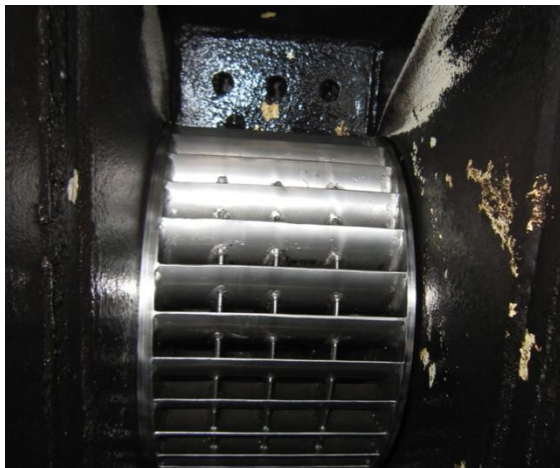
Figure 30: Crossflow runner viewed from below turbine. Still in good operational condition after 10 years continuous operation.
