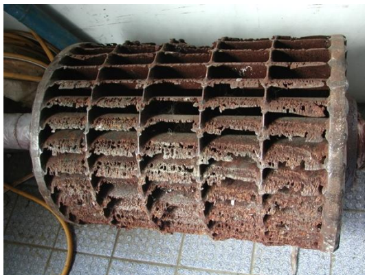
Figure 5: A very badly worn cross flow turbine runner.
