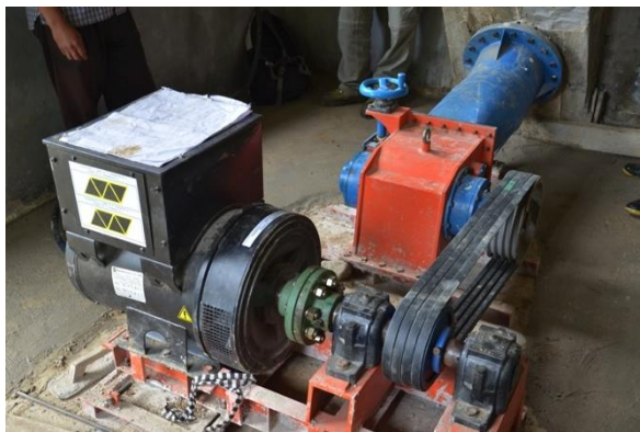
Figure 71: Typical drive belt arrangement showing V belt drive via a secondary lay-shaft with flexible coupling connecting to the generator.
