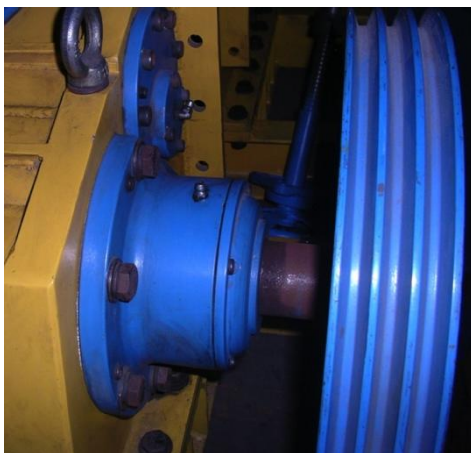
Figure 22: Sidewall mounted runner shaft bearing housing on a cross flow turbine. The grease nipple is visible on the top of the housing.
