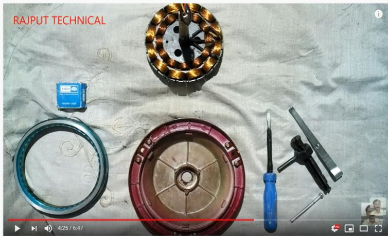
How to change Top end cover Ball Bearing of Ceiling Fan
