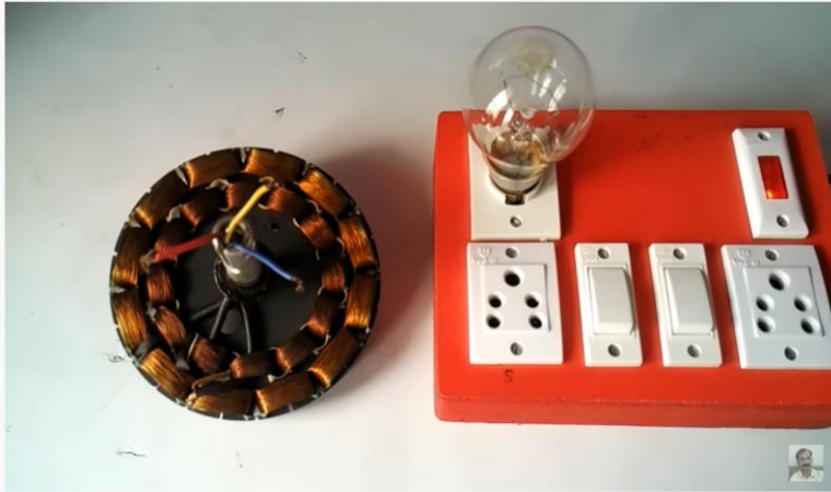
How to check Ceiling Fan Winding with Series Testing Board
