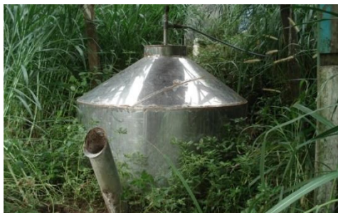
Steel Biogas Digester – Indonesia
